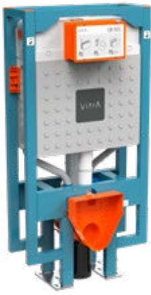
Slim wall-hung frame, 8cm, back-to-back fixation with electrical connection, 3/6 litre H: 1120mm W: 555mm P: 200mm
